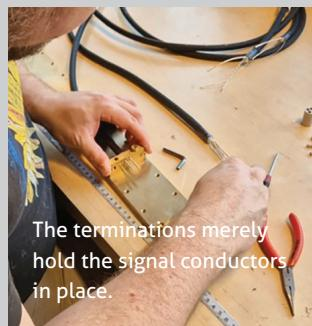
The terminations merely hold the signal conductors in place.
